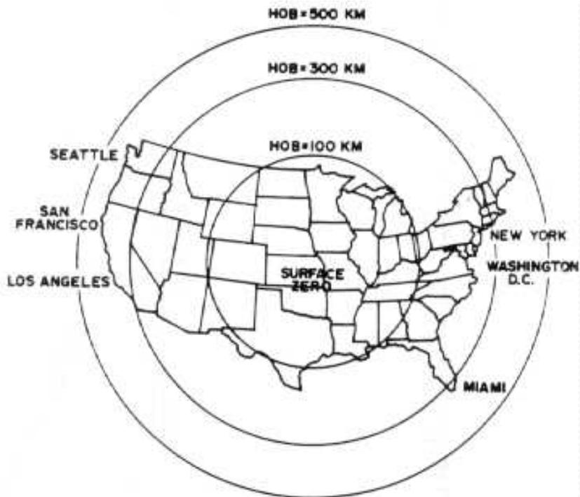
Figure 8-3. HEMP ground coverage for bursts of various heights above the United States. (Source: ref 8-14)
