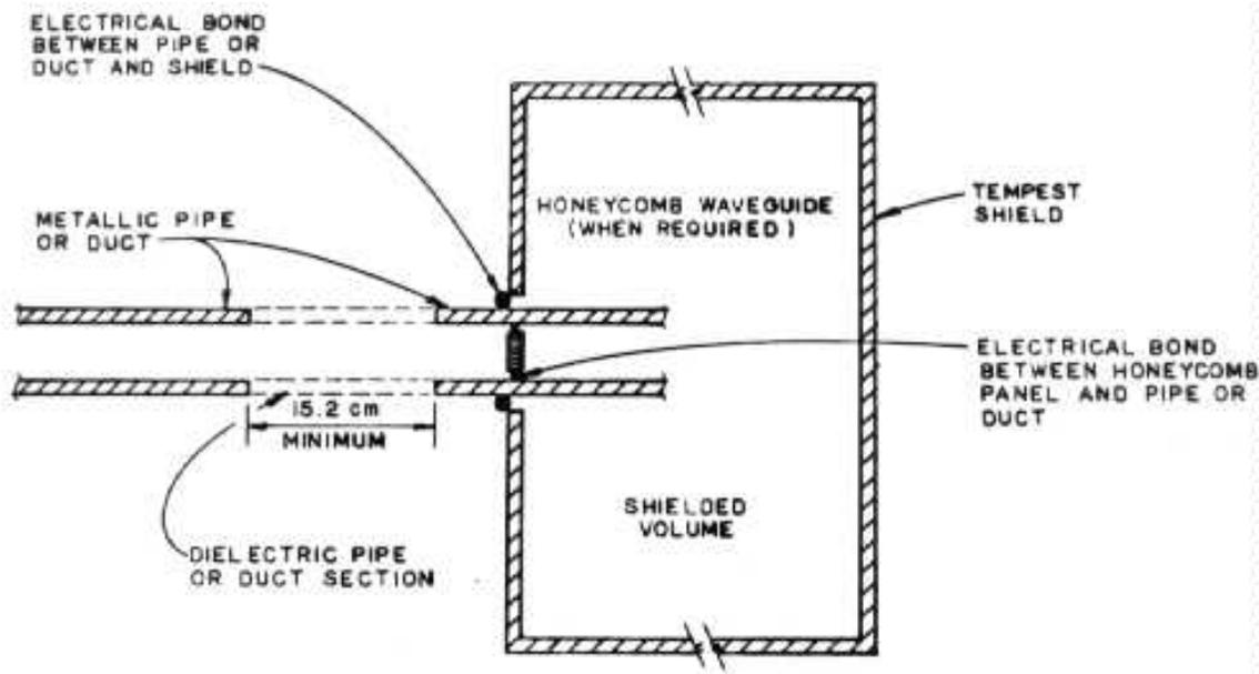
Figure 8-5. Fifty-decibel (nominal) TEMPEST pipe or air duct penetration design.
